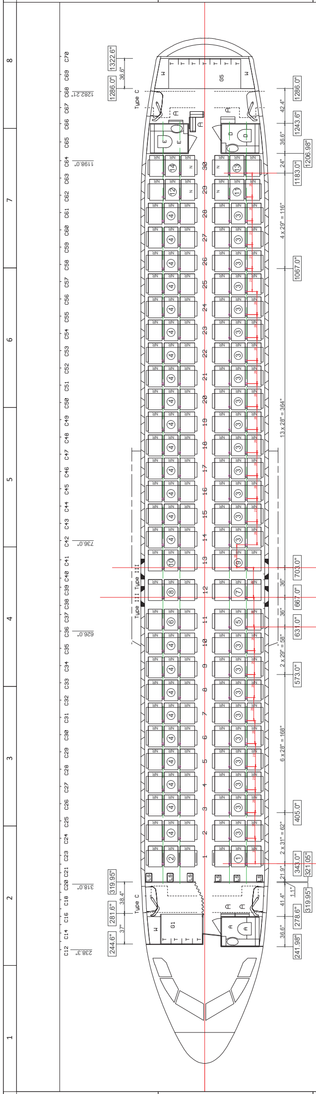
FIGURE 2-E1. LAYOUT OF PASSENGER ACCOMMODATIONS
